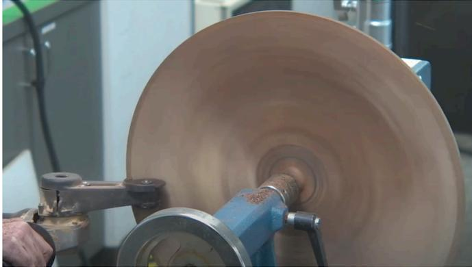
Scott textured the platter face using a mini grinder with a 2-tooth circular blade. He used the tool rest as a guide to steady the grinder. Lathe speed was set at about 400 rpm, but it depends on material, tool and handling..
