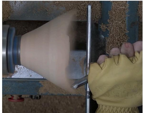
Shaping the "bowl" part of the Three Corner Box. Note the pen marks on the tool rest to help reference the location of the corners. Similar in concept as live edge turning.
