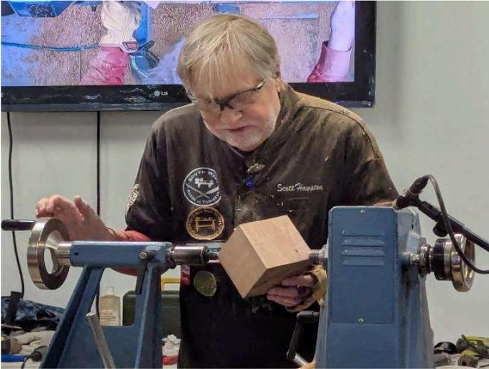
Three corner box starts from a cube-shaped blank mounted on its diagonal axis.
